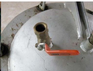
Turn valve to let out air for 10 mins
