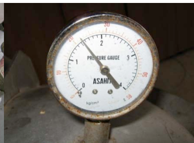
Steam under pressure of 21 pounds for 60 mins
