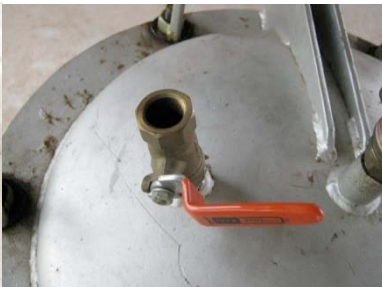
Turn valve on, let out air for 10 min
