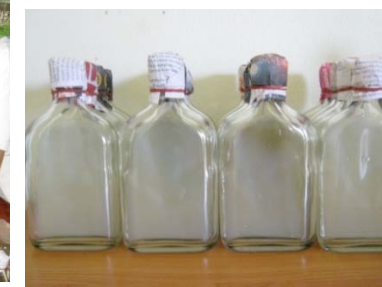
Steam under the pressure at 21 pounds for 30 min
